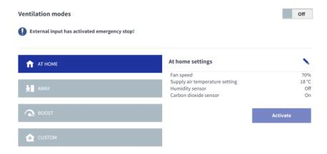
The ventilation unit is turned on and off from the Ventilation Modes menu. If the ventilation unit is turned off, the fan icon will not be displayed (see image above).
